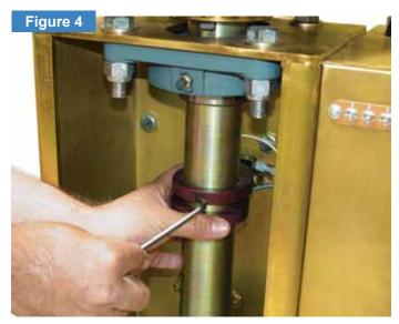
Gate travel is adjusted by loosening the limit Cams and adjusting them until proper gate travel has been achieved.
